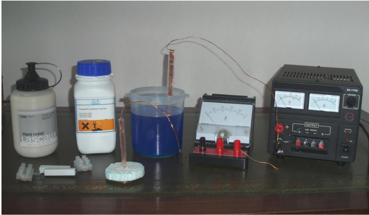
**Figure 7. The Set-Up for Electro-Etching**
