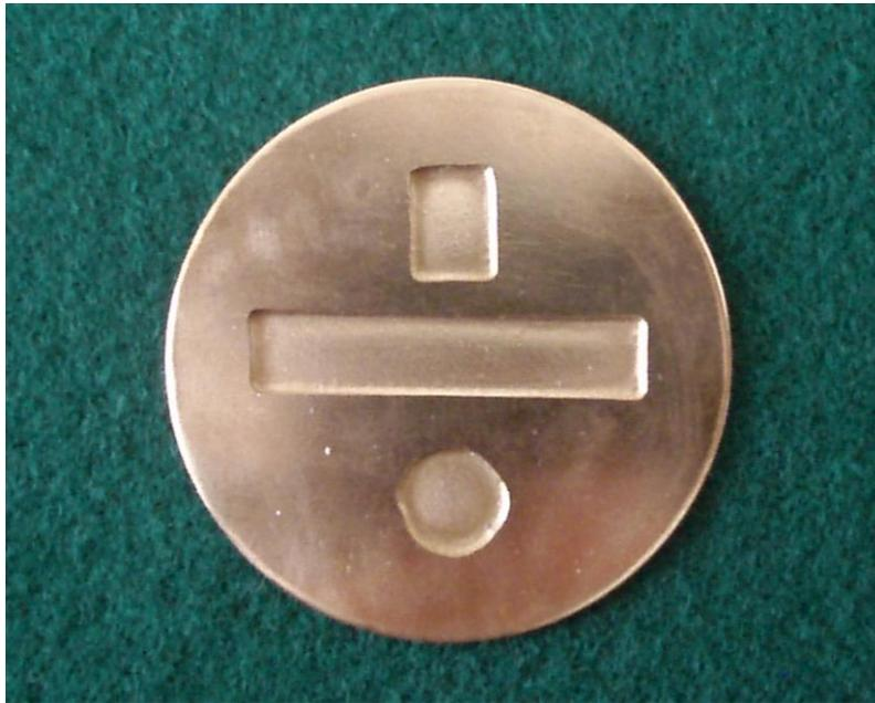
**Figure 10. Test to Show variation in Depth of Etch**
