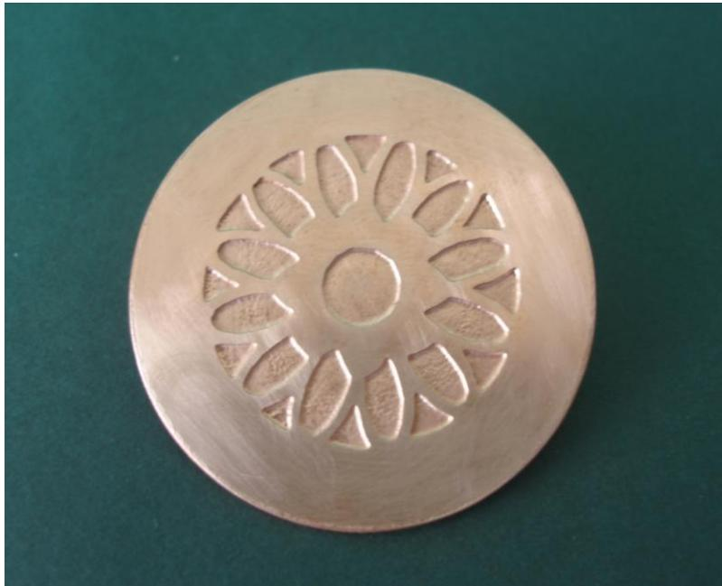
**Figure 8. Copper Sample Electro-Etched**
