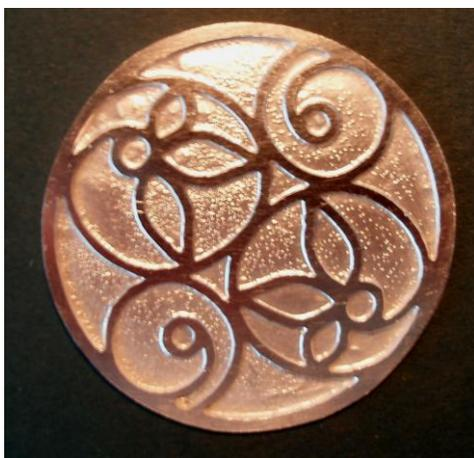
**Figure 13. Sterling Silver Piece Electro-etched in Dilute Nitric Acid**
