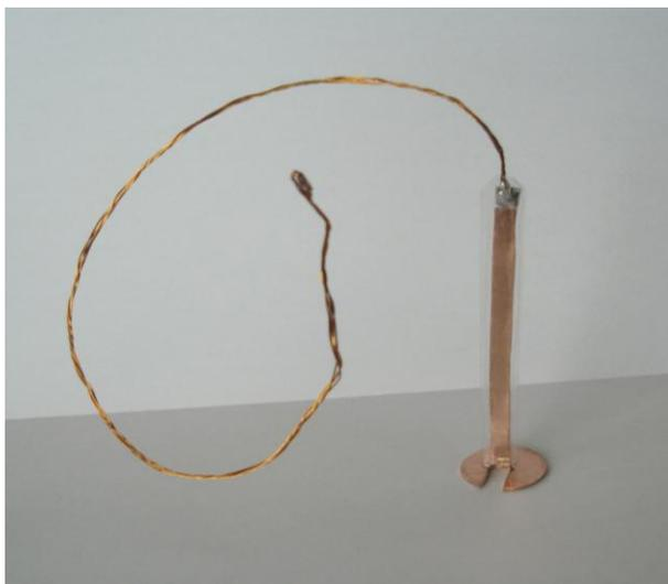
**Figure 3. Back Plate Connector**
