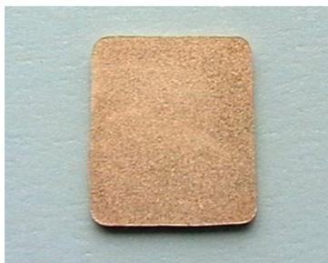
**Figure 7. Fine Grain Structure Produced by Bright Dip**
