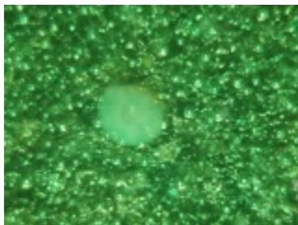
**Figure 17. Magnified View of Imperfection in a Green Transparent Enamel**
